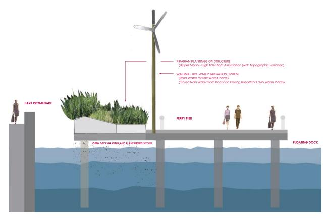
The planted boxes have elevated and low areas mimicking a natural river slope. An artificial irrigation system pumps river water into the boxes.
